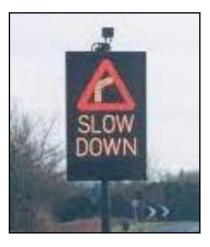
This is a VAS (Vehicle activate sign). In this example the sign is also activated by the speed of a vehicle but rather than presenting feedback to the driver it illuminates (when triggered) a standard traffic sign to warn the driver of an upcoming hazard
